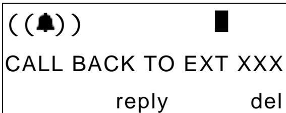
6. Lift the handset or press *reply* to activate the Call Back.
