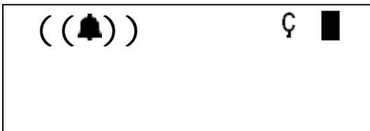
When the handset is in the key lock mode, and you press and hold the *Trans* key, the LCD displays the following message for three seconds.
