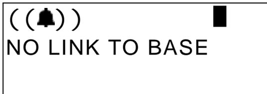
The user must get closer to the base, or check the base power status. The user can also try to re-register the handset to check the registration status.
