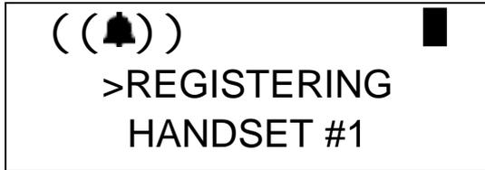
*Note:* Up to two line cords can be used to connect two digital station ports from the KSU to the two jacks on the base. If the handset ID is #1 this means the handset is connected to Line #1. If the handset ID is #2 this means the handset is connected to line #2.
