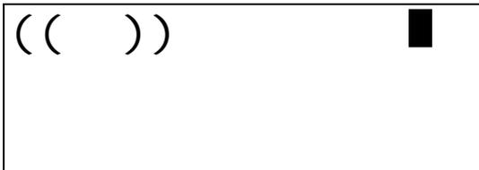
If you set the status to Ring and Vibrator mode, the phone displays both the ring and vibrator icons on the LCD.
