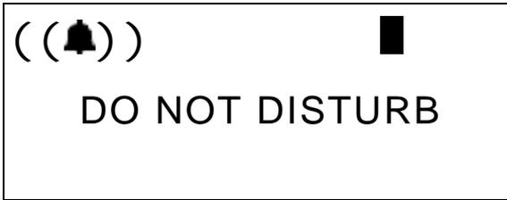
2. When the display reverts back to idle condition, the DND condition shows in the bottom row of the display.
