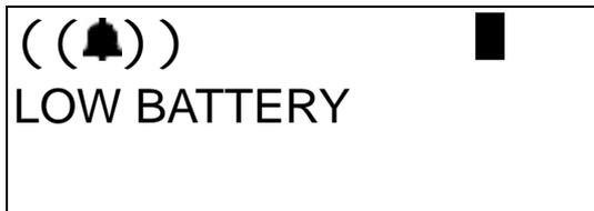
When the battery power is too low, and the handset is not in the standby mode, the phone flashes the icon at the cadence of 0.5 sec on-and-off repeatedly. *Note: The phone does not flash the icon when the handset is in standby mode.* If the handset is in the talk mode, the unit also sounds a warning beep every 15 seconds.
