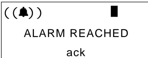
Press the *ack* soft key to stop the alarm, or wait for it to stop automatically.
