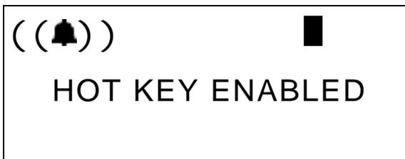
To disable hot key, while the telephone is idle, press *Func* + # + 6. The display momentarily shows the feature status.
