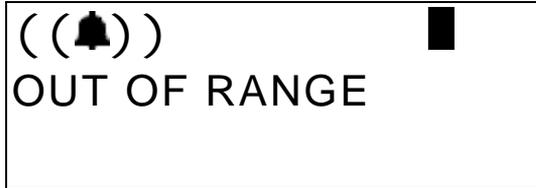
The user must move closer to the base, or the call will be dropped within 30 seconds.
